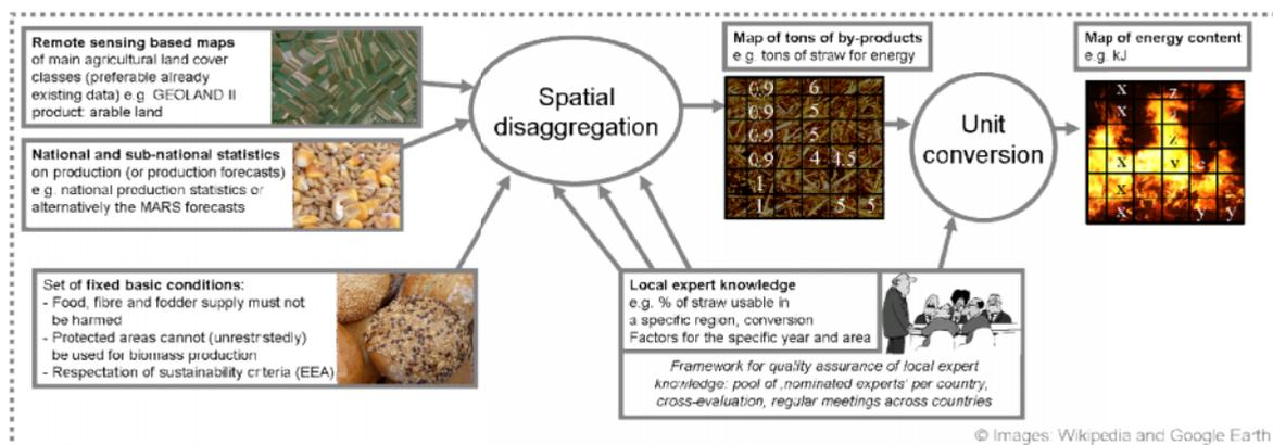
**Figure 1: Simplified approach of using terrestrial and remote sensing data for biomass potential assessment for energy.**
